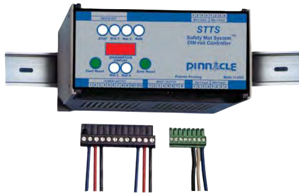
Enclosure mounting: 35mm DIN-rail mountable or mounting screws on corners of enclosure requiring two combo-head screws (3.5 x 0.6 mm x 14 mm or #6 x .5)
