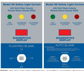
The (RSD) device provides blanking scrolling operator diagnostic message display and system status <u>without</u> entry into the machine control panel. This saves time for lockout/tagout requirements and safeguarding blanking adjustments.
